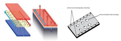
Two-dimensional electron gas between two doted semiconductors (Spot error in picture!) Measure of macroscopic (!) Hall tension
